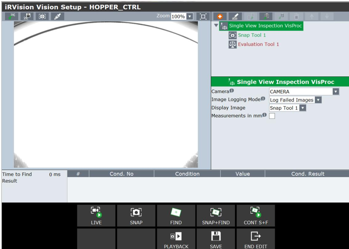
Select "Snap Tool 1" and adjust exposure and resolution; reduced resolution promotes faster control.
