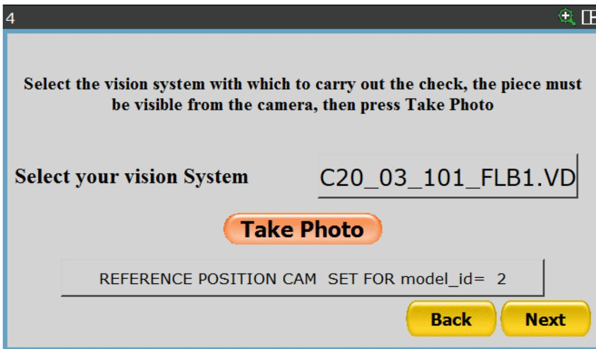
Following the selection of the vision process, it will be possible to press the “Take Photo” button to define the current position of the object as reference position. This function is particularly useful when using the camera to center the object held by the robot gripper. The vision tool must have already been defined.
