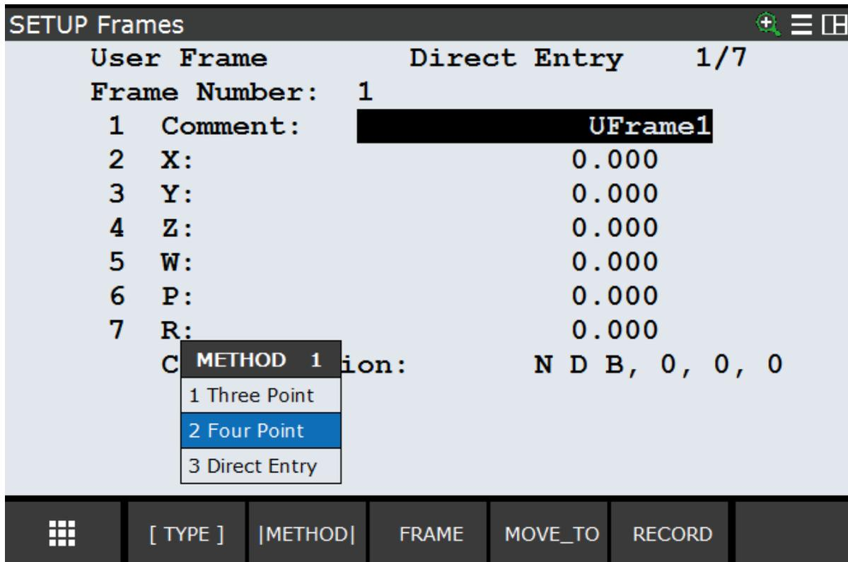
Press "Method" and select "Four Point". Creating a frame with the 4-point method is ideal for creating frames on the calibration grids, whereas the 3-point one can be used to create reference systems for creating pallets, for example. The 4-point method will be shown on the following pages.
