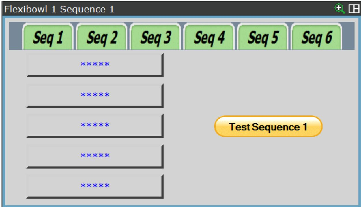
Select the first box of the list and choose the desired movement from it; if necessary, proceed with assigning the second box, so that the desired sequence can be defined.
