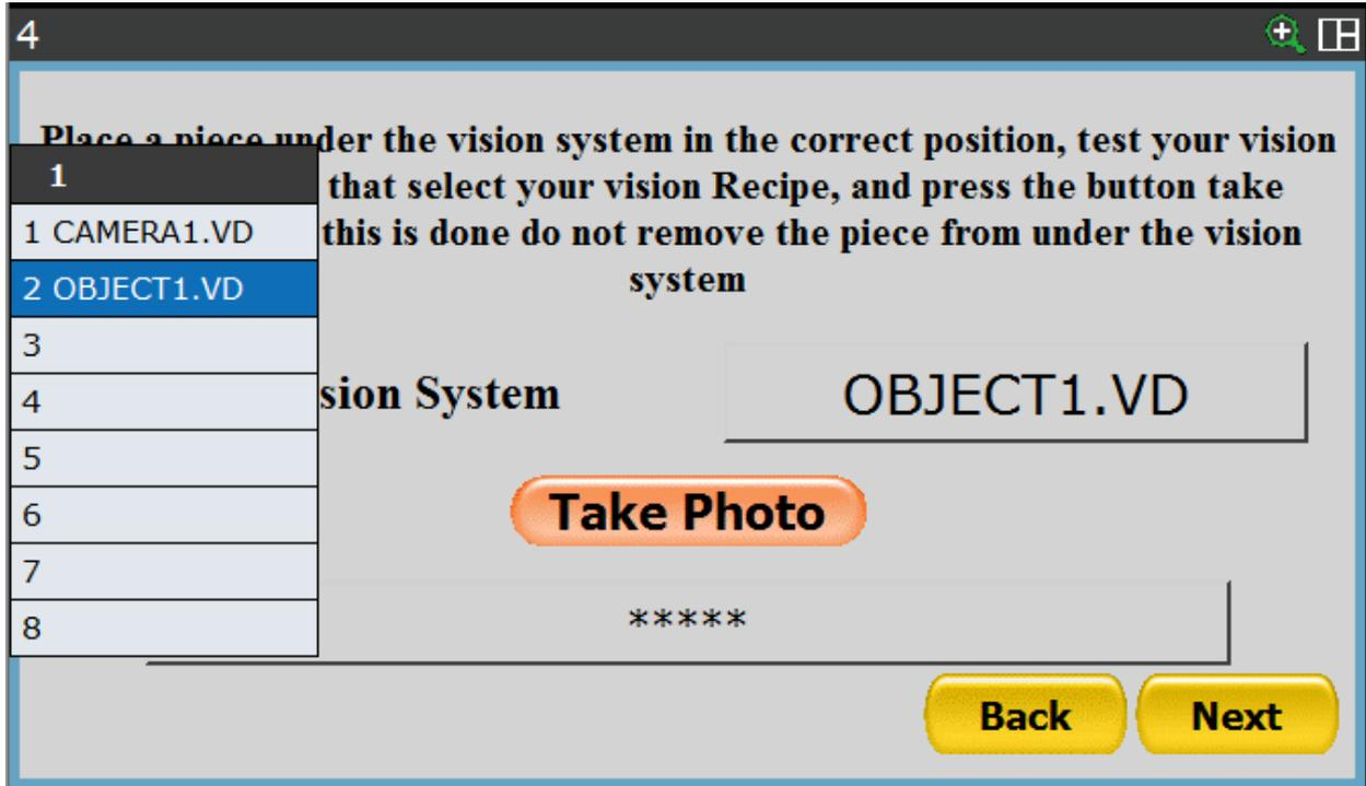
After selecting it, you must place a single piece on the Flexibowl in the vision area. Once the component has been positioned, the robot must be taken out of the way so that the camera can take a photo and identify the position of the piece.
