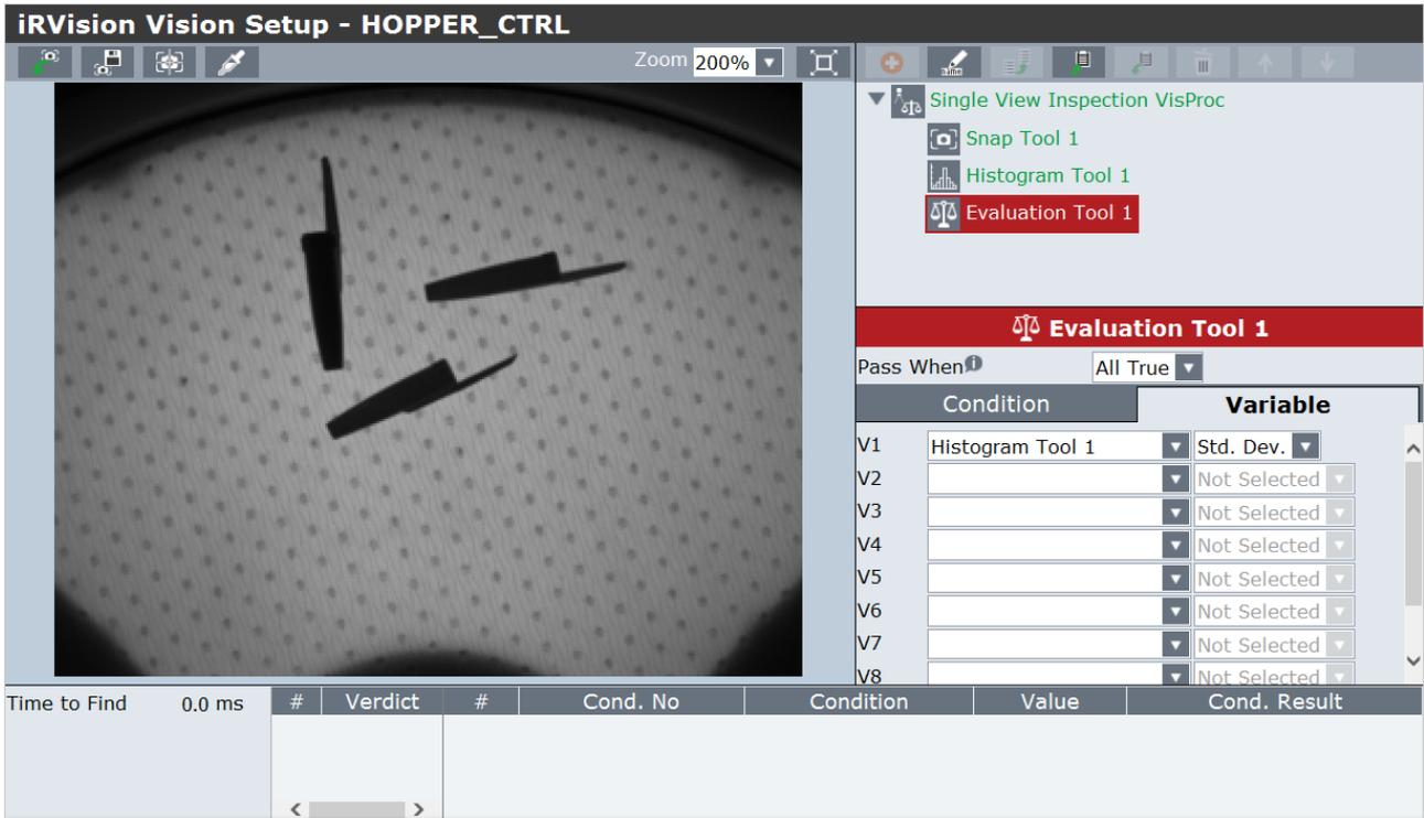
Then select the "Condition" tab and enable the "C1" condition: the control will only be successful if variable C1 is less than a constant, which specifies the threshold value.
