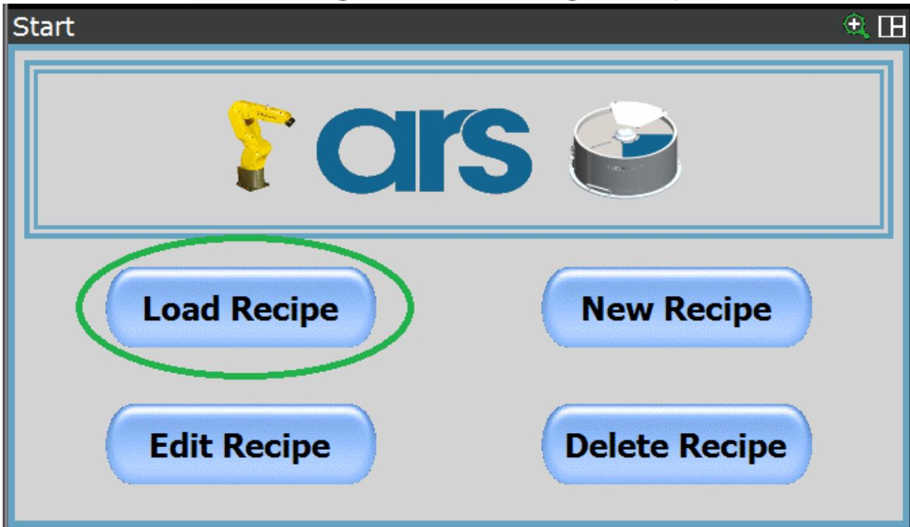
A recipe can be loaded manually without having to retrieve it from an external device.
