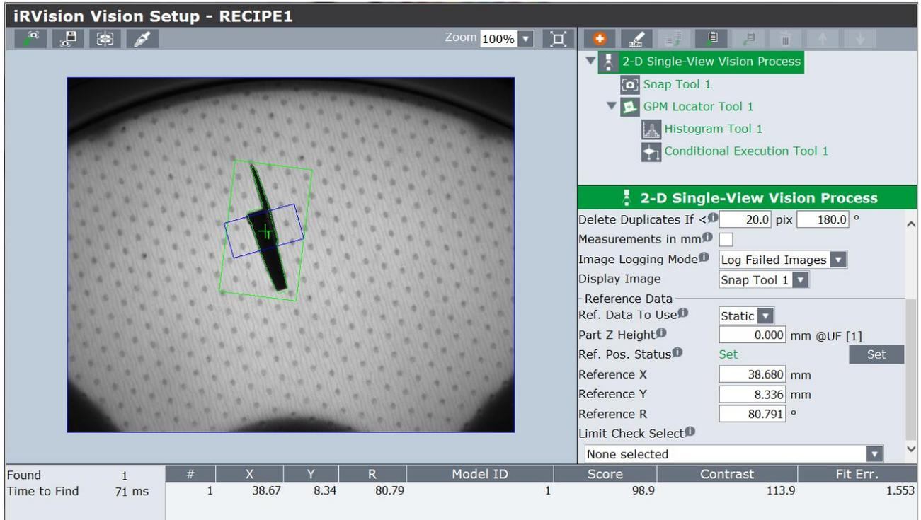
Place another piece close to the part to be picked up and repeat the photo with the “Snap+Find” button; the vision system must discard the object.
