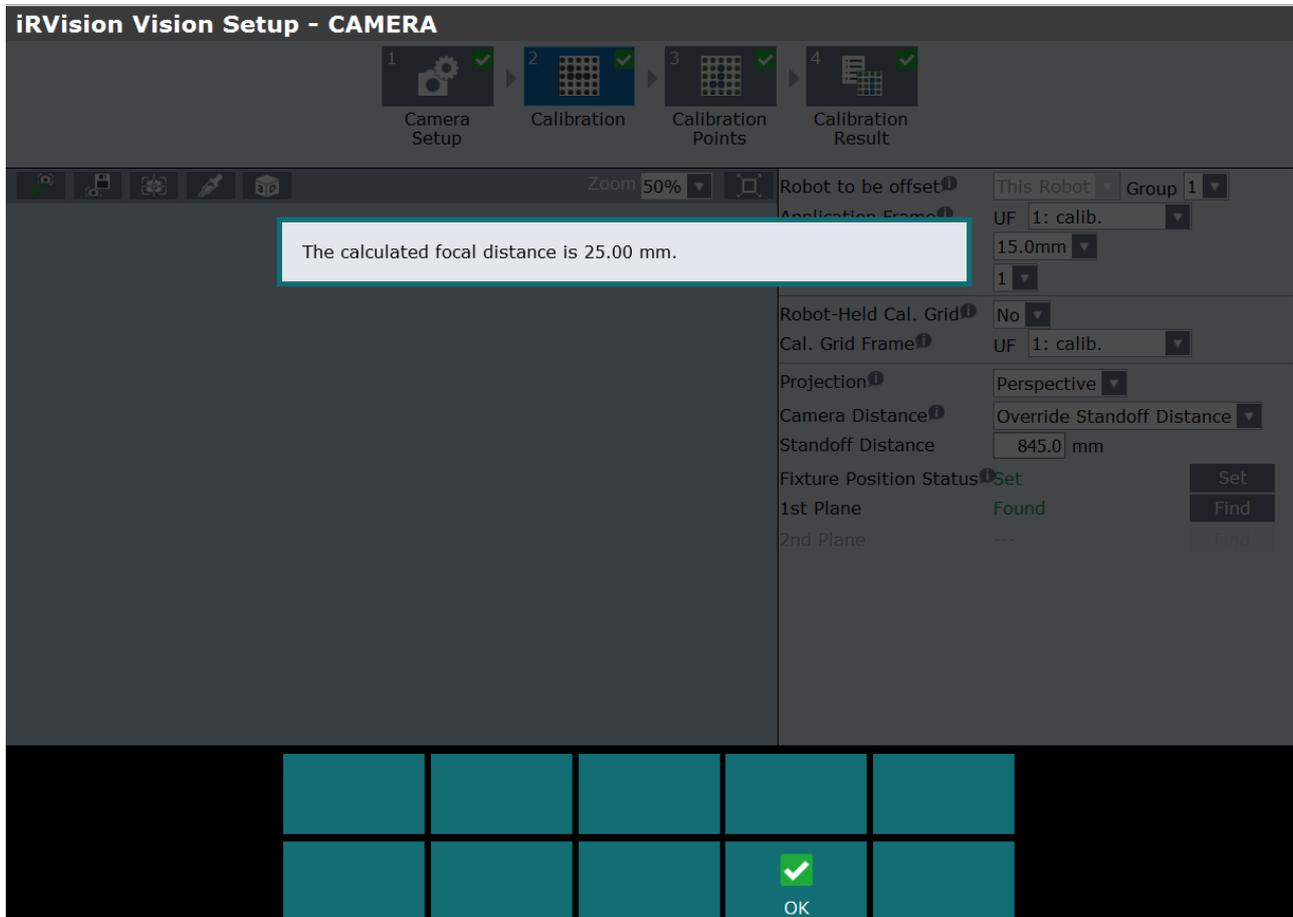
If the data entered are correct, the data relating to the focal length of the lens used will be given. It is important to compare this data with the actual one of the lens used; if there are significant differences, check the entered data.
