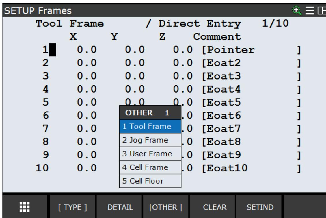
Press "Detail" to access the Tool configuration parameters
