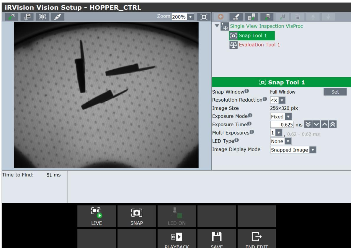
Select the “Single View Inspection VisProc” main vision process and press the red “+” button to add the control “Histogram Tool”.
