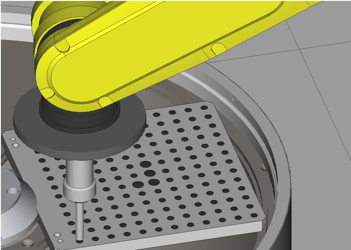
Move the robot to the last position (System Origin) and also record this last one.
