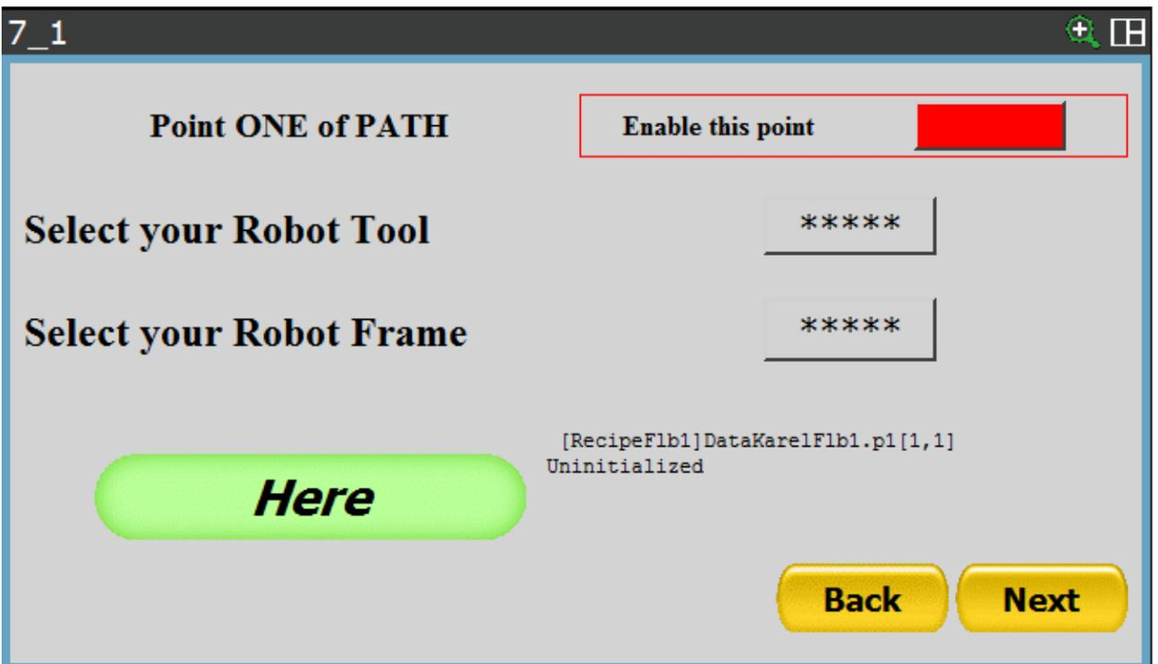
Enable the passage point using the relevant button found at the top right.
