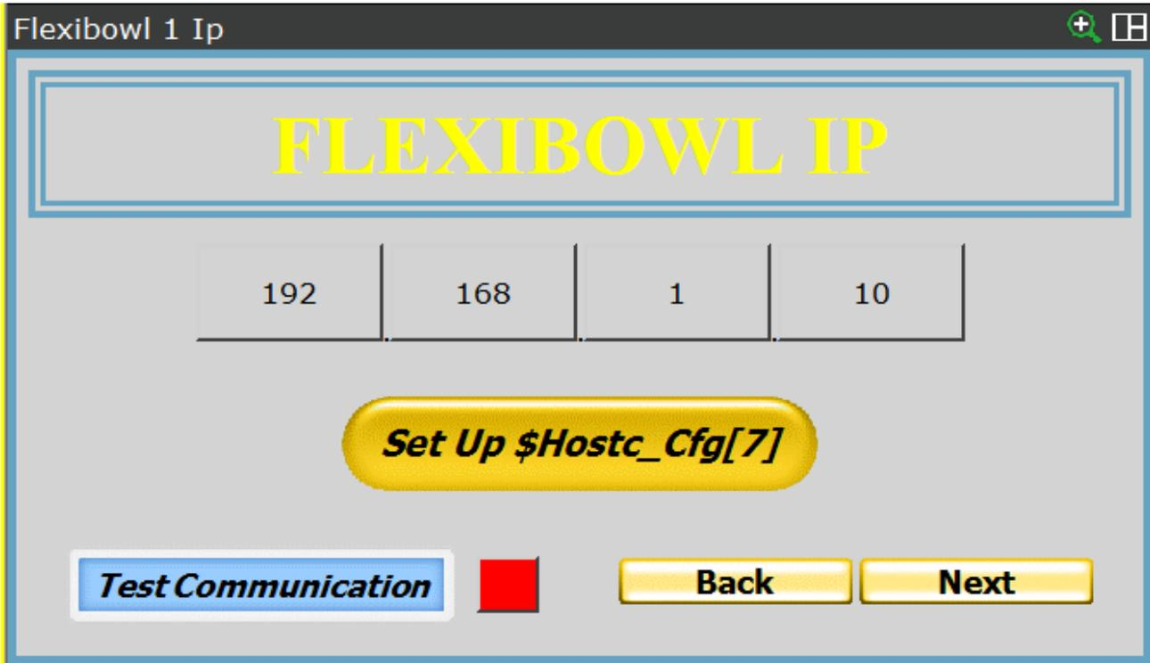
Once you have inserted the correct IP address, press “Set Up \$Hostc\_Cfg[7]” to configurate the communication client “C7”. During the configuration of FlexiBowl 2, client “C8” will be set.
