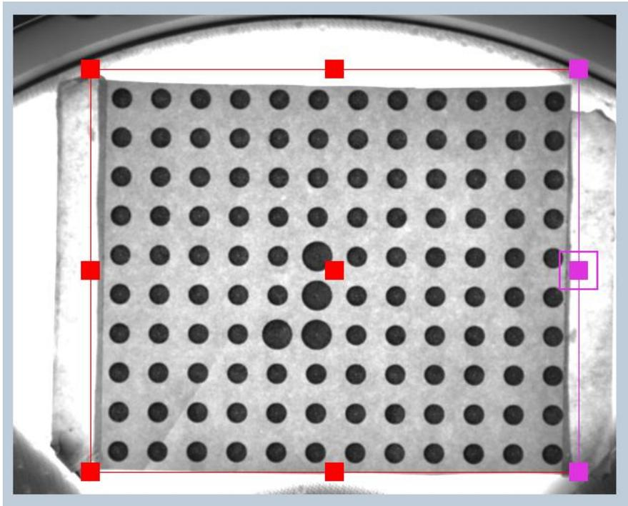
The vision system will identify all the circles it will be able to recognise, with a cross reference. For optimal calibration, all the points on the grid must be recognised.
