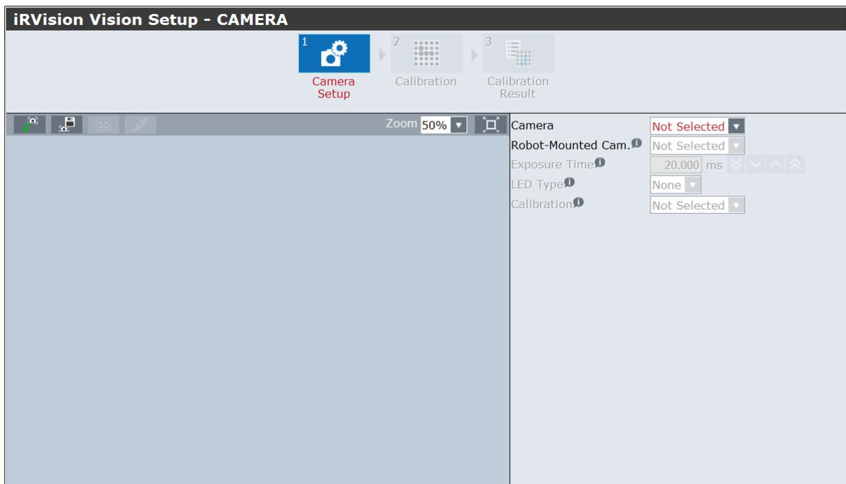
Place the calibration grid in line with the Flexibowl pick-up area and complete the fields on the right side of the page.
