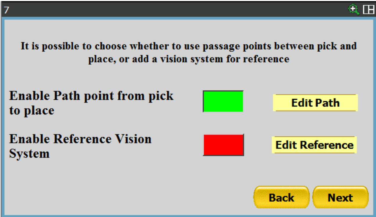
With the following procedure you can add up to 10 intermediate points, related to a particular model.
