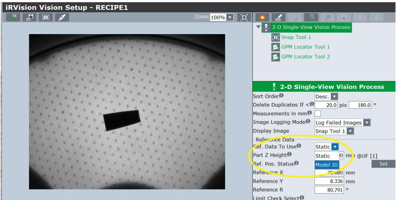
Press the “+” button to add a new line associated to model 2
