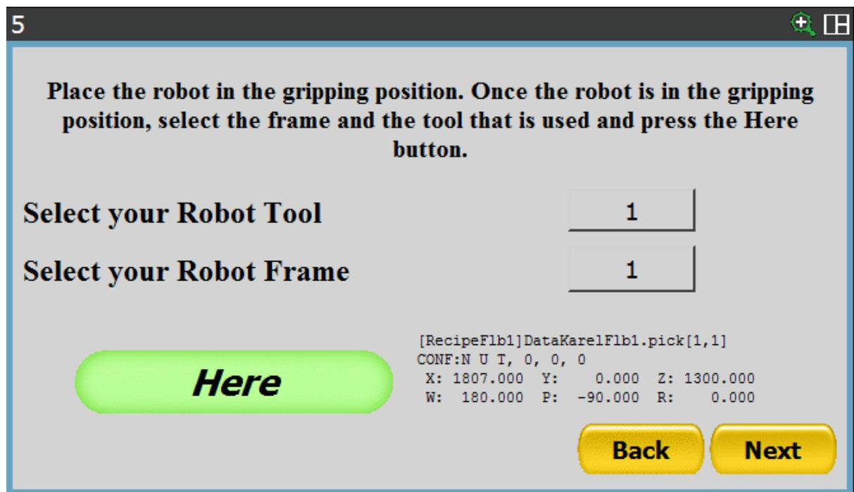
Then bring the robot to the final pick-up point and press the “Here” button to record the pick-up point. Then press “Next” to proceed.
