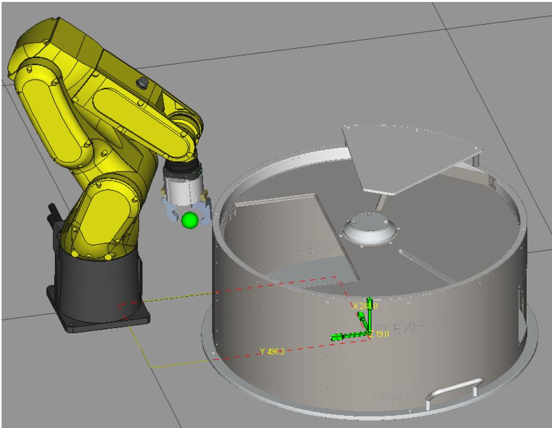
To record the first point, move the cursor over the “Basic Vertex” item and press the “Record” button together with the “Shift” button on the keyboard.
