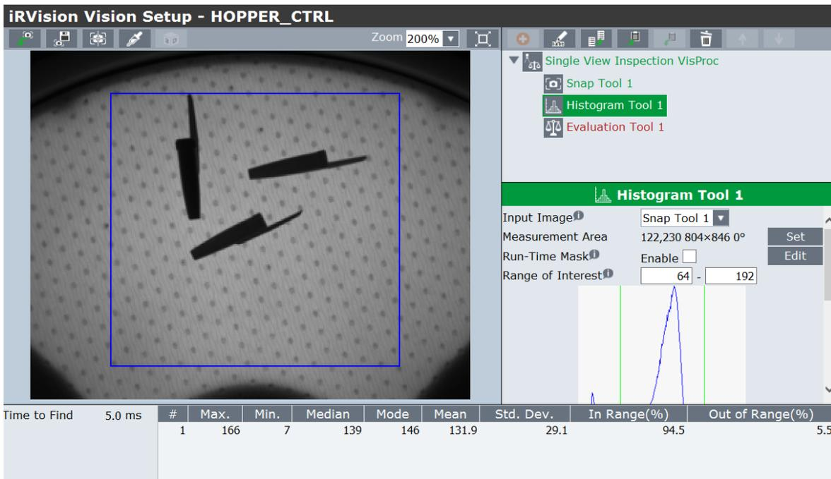
Pressing "Snap+Find" shows the values relating to the image; the value that can be used is the "Std.Dev." Assuming that you will consider the Flexibowl area as filled correctly with more than 3 pieces, the threshold value you will use is 28.
