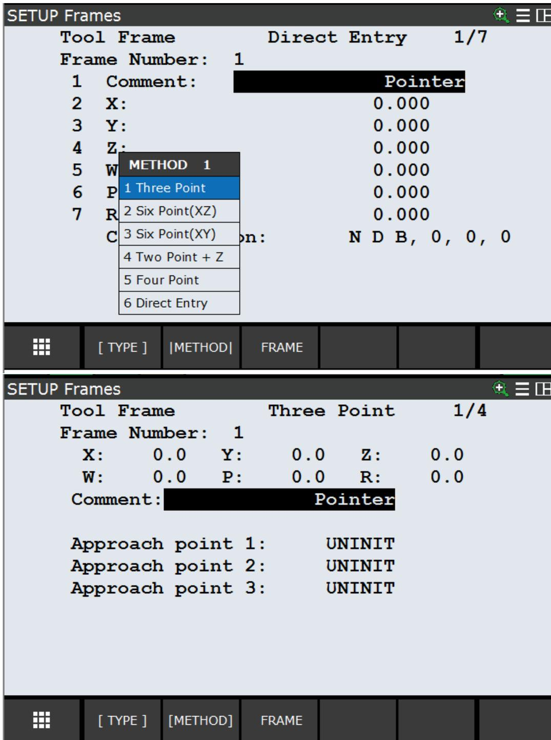
Use the three-point method to set the tool reference system. The three points must be memorised in reference to a common point with three approaches from different positions. As a result, the tool centre position is calculated.
