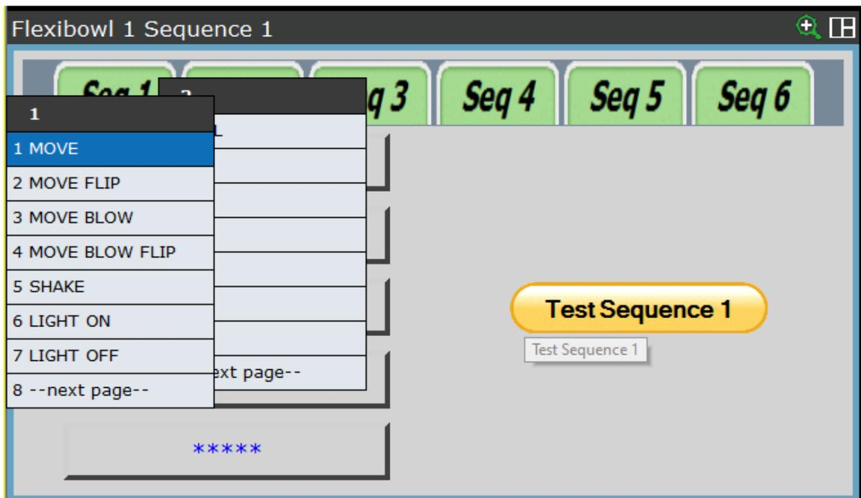
It is possible to verify if the sequence works by using the button “Test Sequence”
