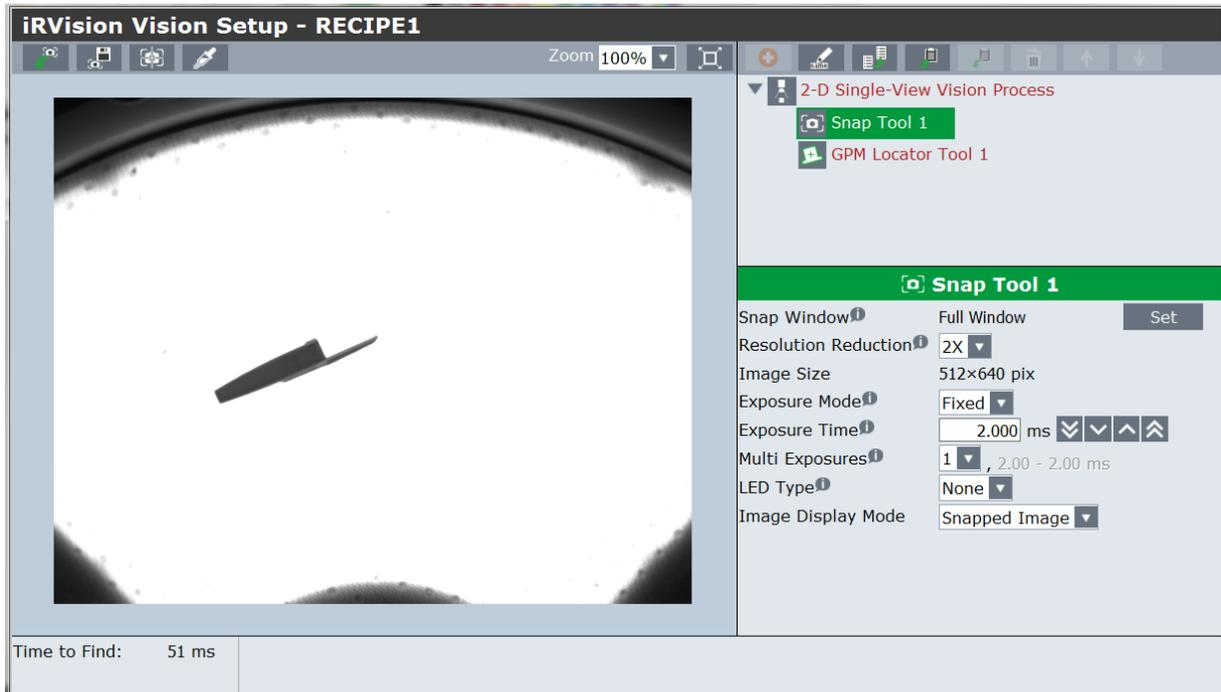
From this page, you can adjust the exposure time of the image and the resolution you want to work on; the higher the resolution, the longer the processing time.
