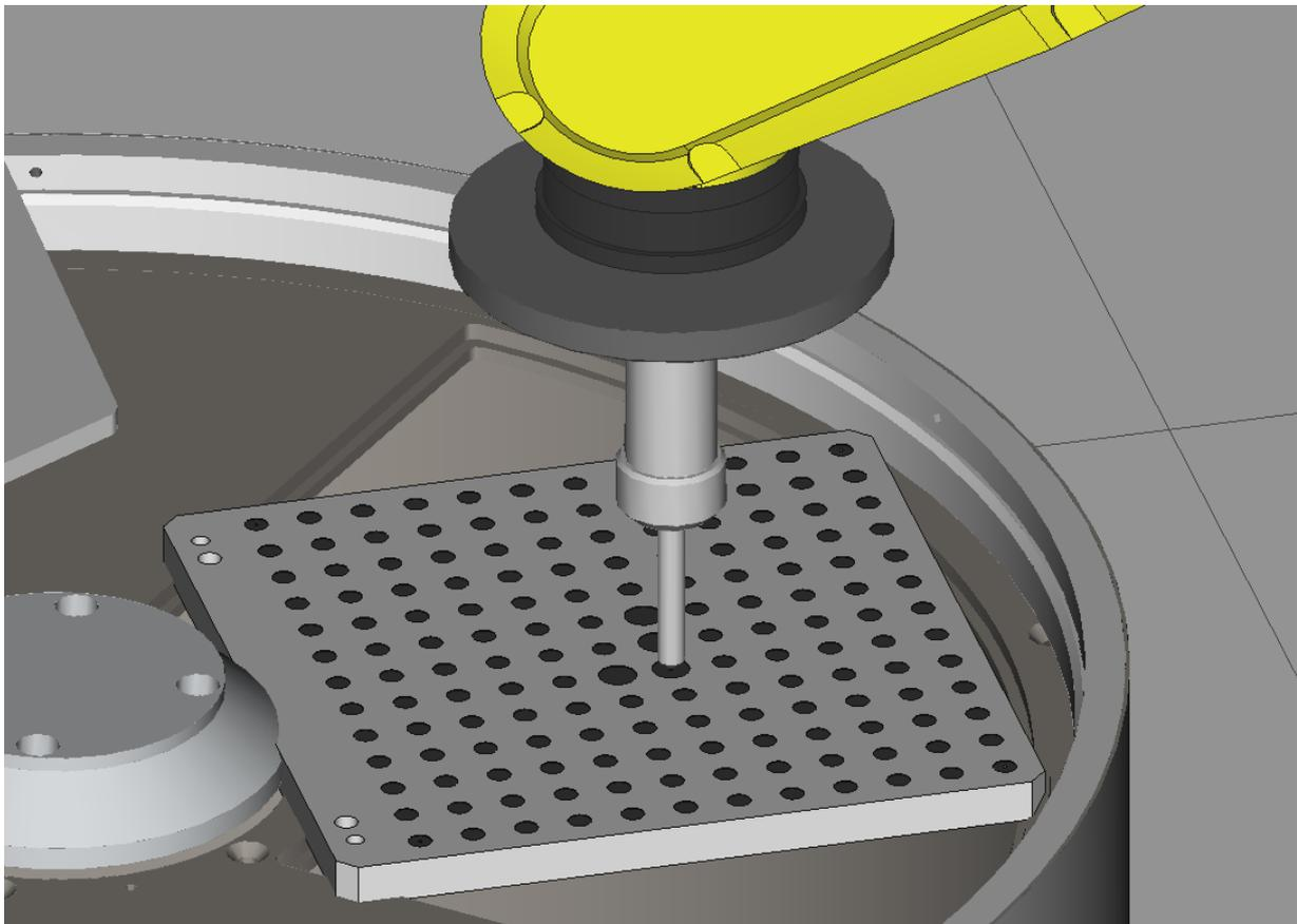
After saving all 4 points, the Frame will be calculated and the XYZWPR values referring to the robot base will be written.
