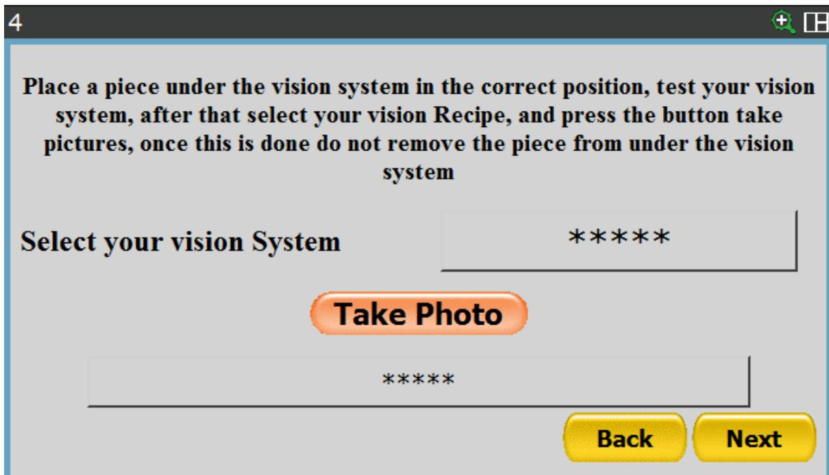
After clicking the header box with \*\*\*\*\* you can select the vision process from the drop-down menu, which you want to associate with the recipe being created.
