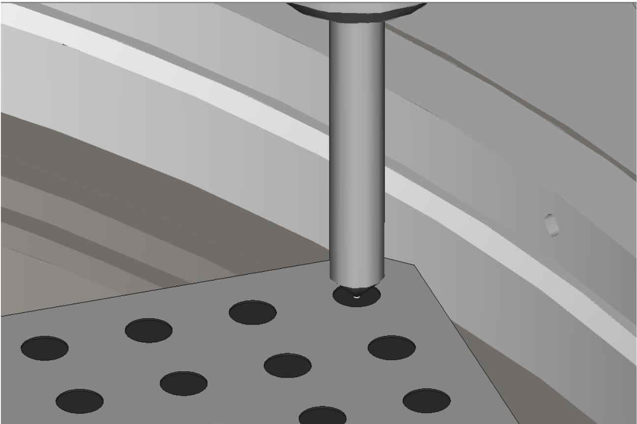
Move the robot to the third position (Y Direction Point) and record this position.
