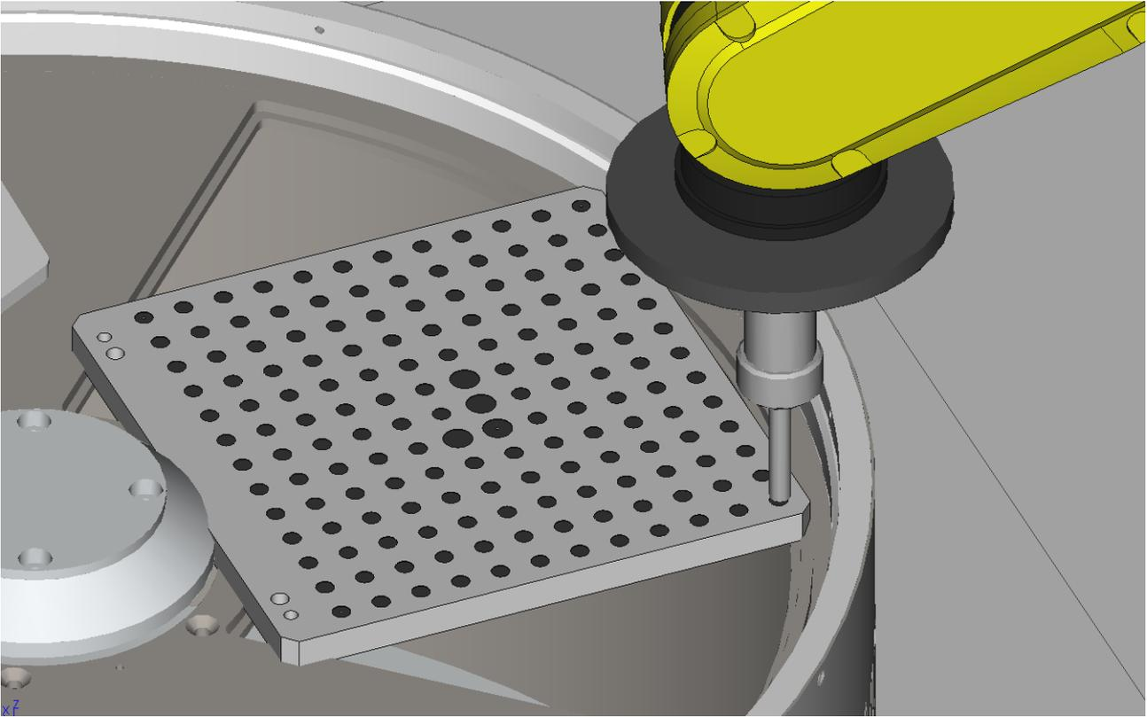
Then select the first point (Orient Origin Point) and press “Shift” + “Record” to save the position.
