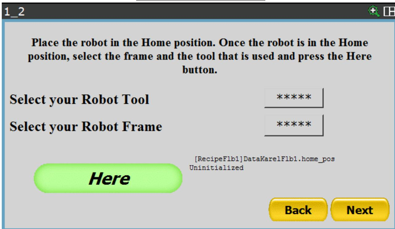
The page that will be shown allows the “Home” point to be recorded as well as the starting or resting position of the robot. The number of the Tool and that of the Frame which the position will refer to must be set so as to record this position.
