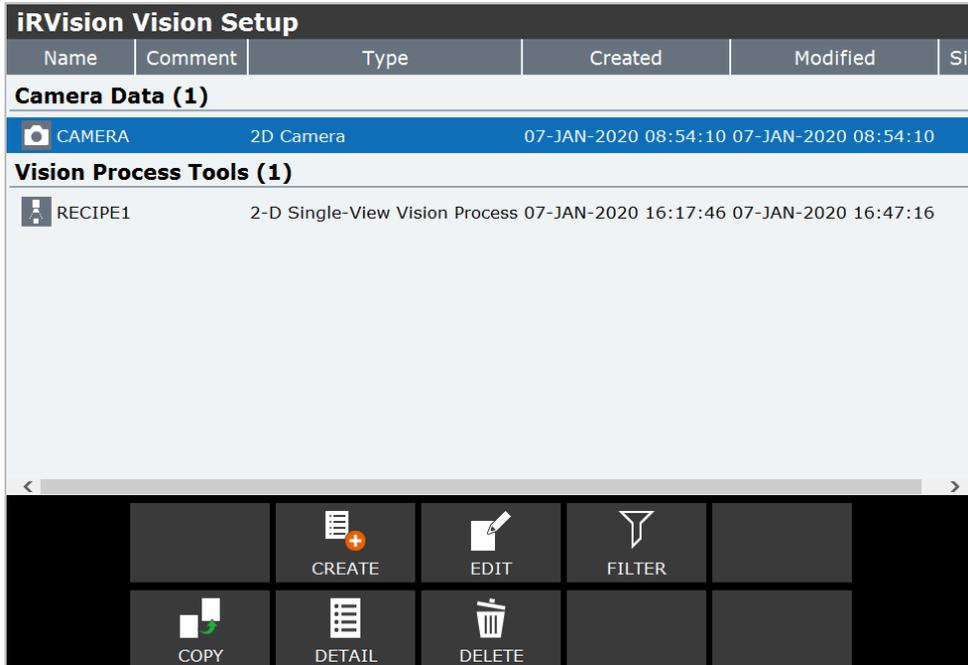
Use the “Create” button to add the vision process required for the control
