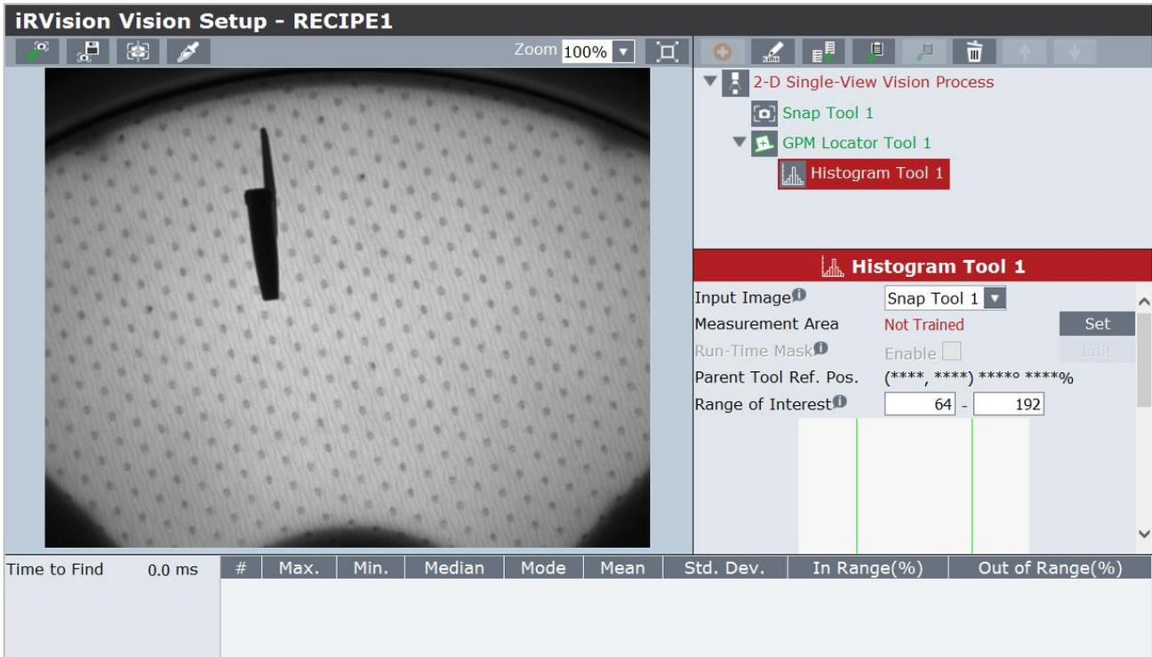
Press “Set” and define the control area; this area must correspond to the overall dimensions of the grippers.
