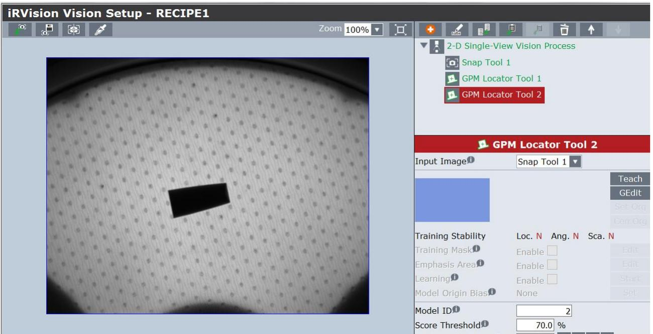
In this example, a model of a different component will be created but the procedure is the same even if 2 models must be created, associated with 2 different sides of the same piece.
