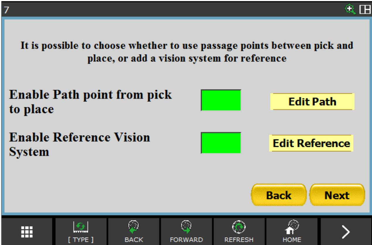
Enable the option “Enable Reference Vision System” by using the dedicated button placed next to the entry “Edit Reference”. Once you have selected the option, it will be possible to access the relative menus, then press the button “Edit Reference”.
