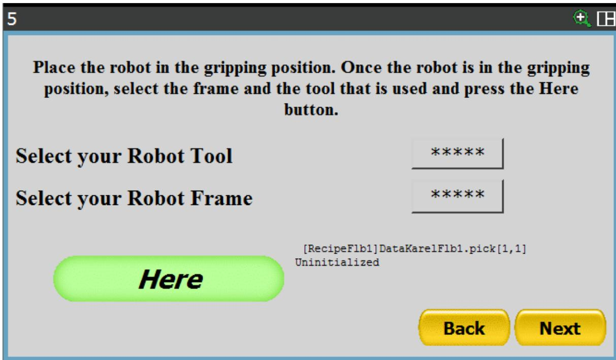
Just like the previously seen point recording pages, this page also offers the option of setting Tool and Frame.
