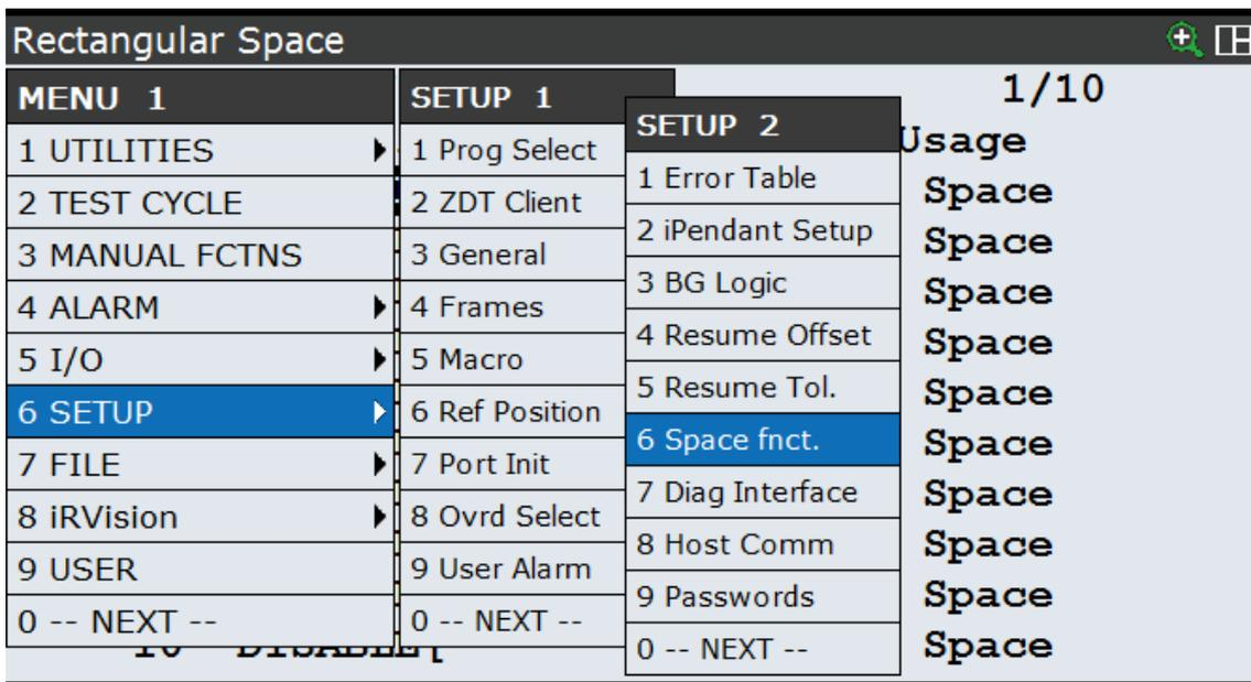
Select the desired space function and press the “Detail” button to configure it
