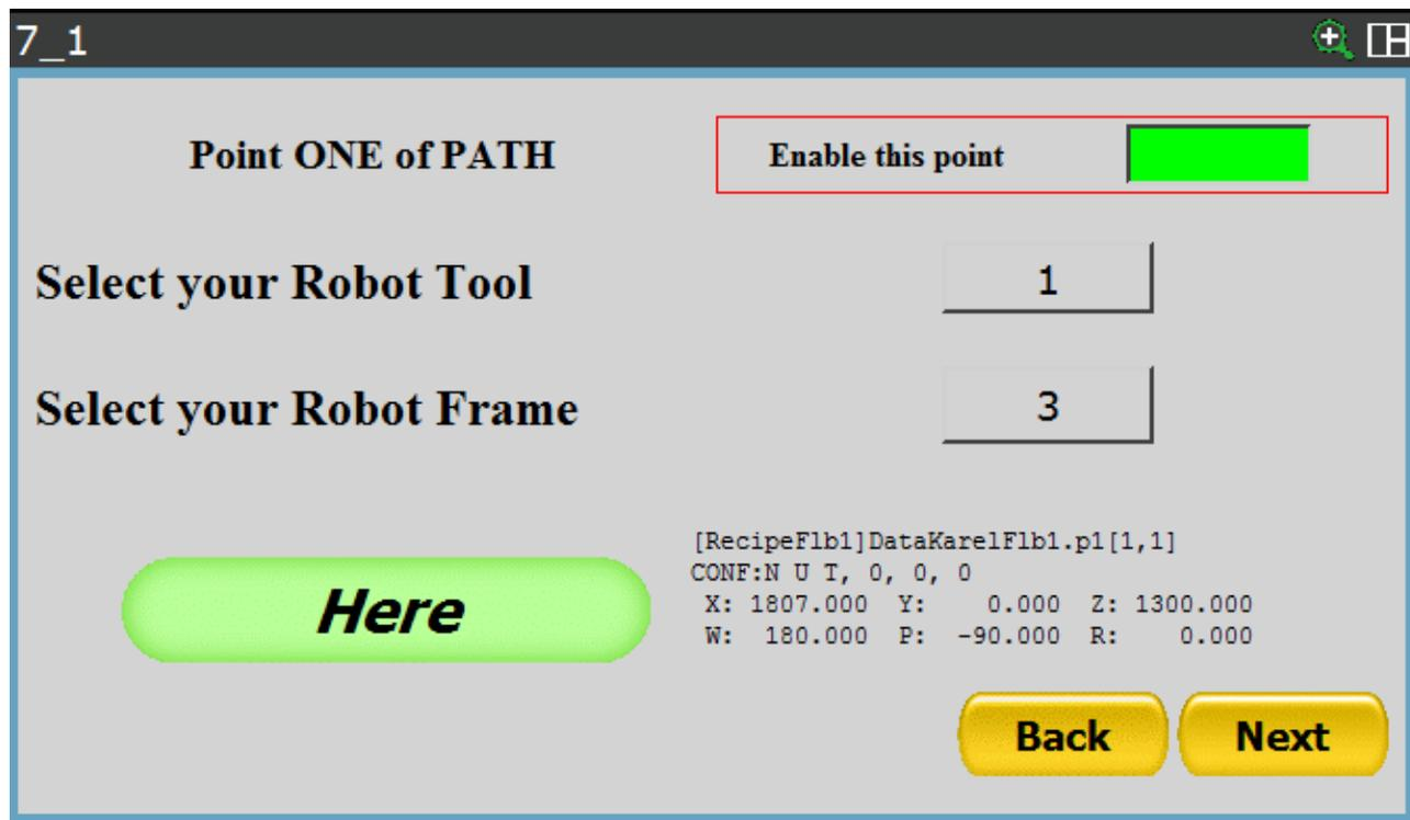
With the same procedure, the following pages allow you to enter up to 10 passage points for the robot.
