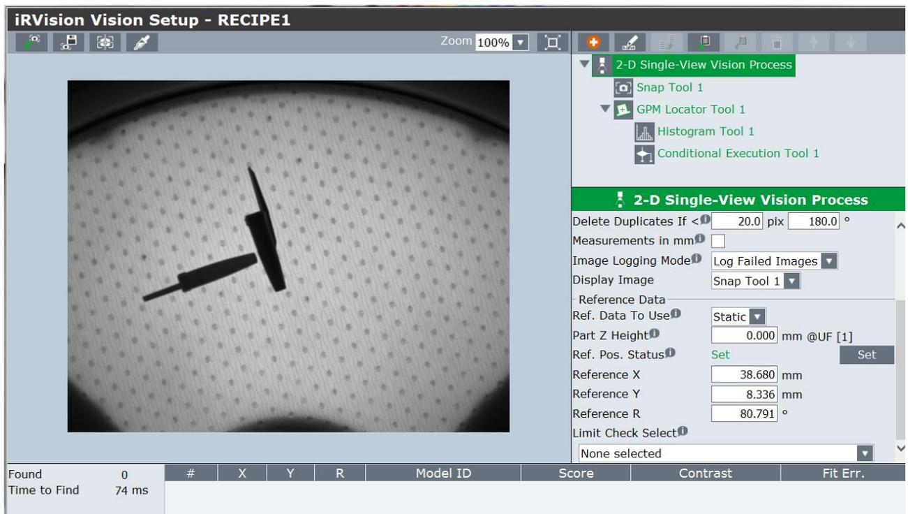
Check by selecting the “Histogram Tool 1” tool and press “Snap+Find”.
