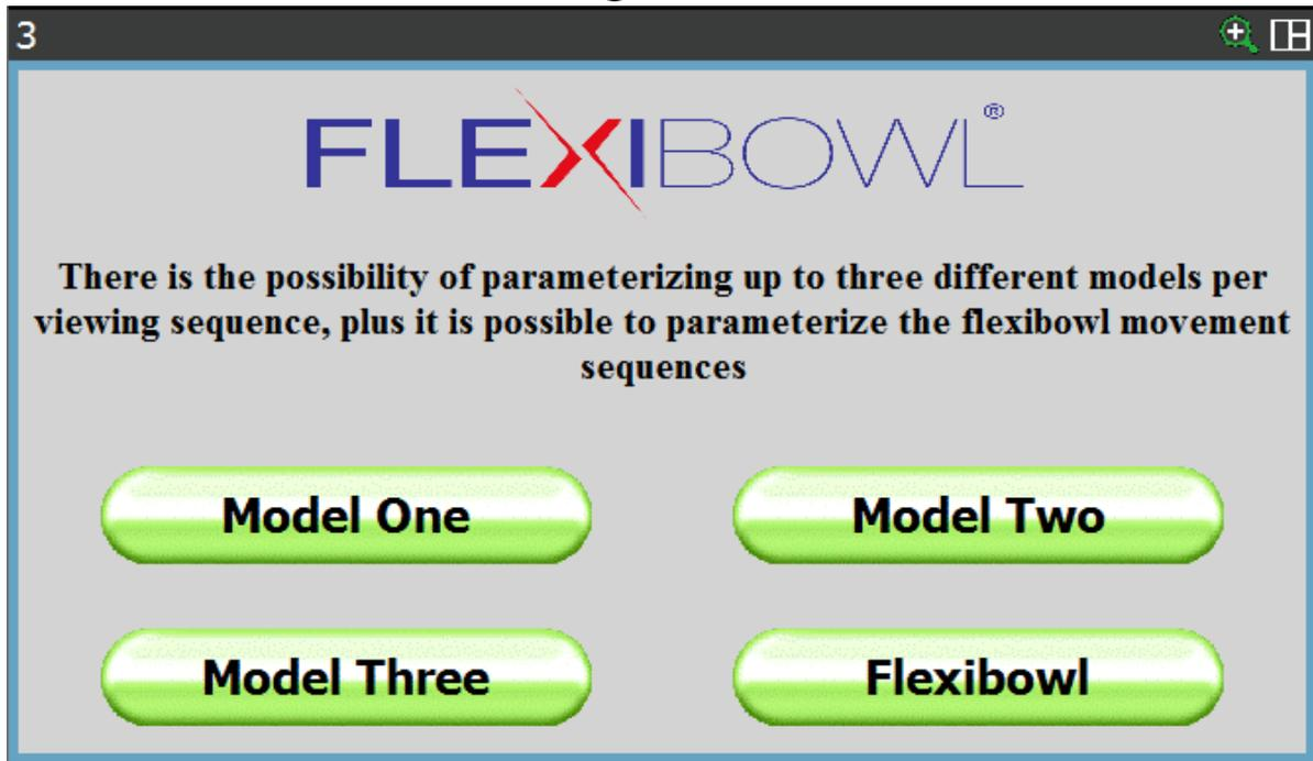
Assuming you must develop an application where the robot picks up a piece from a Flexibowl in a single position, item "Model One" must be selected.
