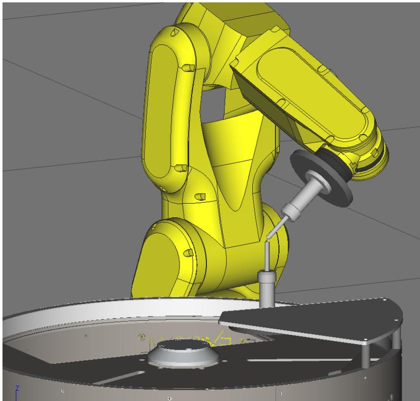
To record the points described above, you must select the desired point by moving the cursor to it and then pressing “Shift” and “Record” simultaneously.
