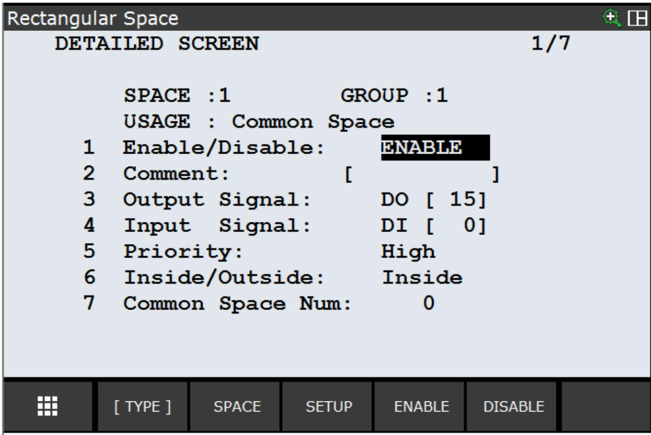
Enable the “Space Function” by pressing “Enable”.
