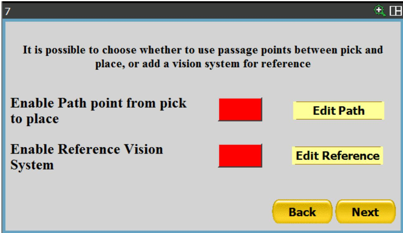
On this screen you can choose whether to enable or not the introduction of intermediate passage points between the pick and place phases.
