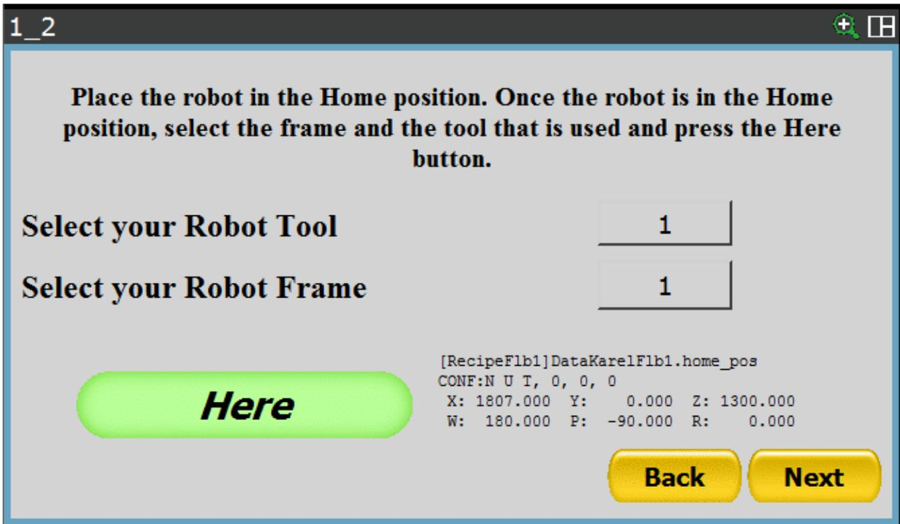
Once both the Tool and Frame have been set, you must move the robot to the desired position and then press the “Here” button. The Cartesian coordinates that describe the “Home” position will be displayed on the right.
