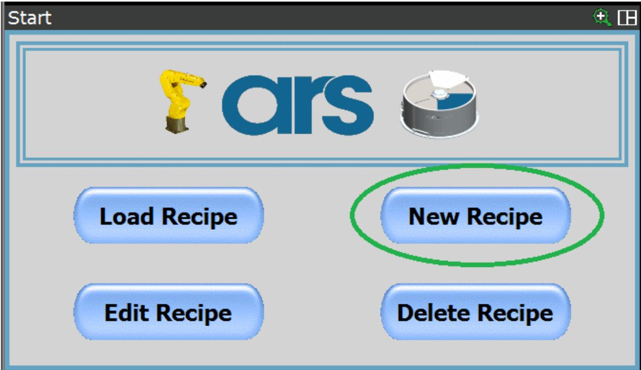
Use the “New Recipe” button, found on the first page of the interface, to access the submenus for creating a new recipe and therefore, a new product to be processed.
