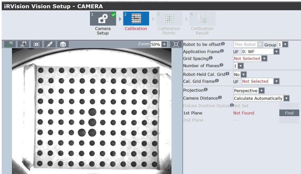
**Application Frame:** set the User Frame number that will be recorded on the calibration grid.
