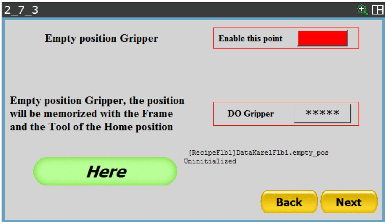
The page that will be shown allows the “Empty Gripper” point to be recorded as well as the emptying position in a given area. In order to record this position, you must only set the signal that will be reset once it reaches the position.
