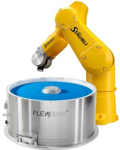
This Plugin was developed with the idea of communicating quickly and safely with FlexiBowl® through **STAUBLI** robots by using instructions in VAL3.
